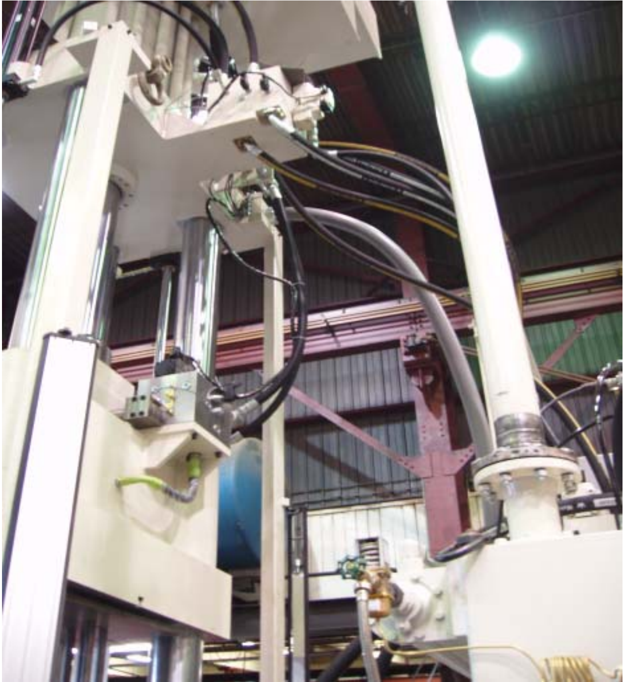
Rear view of press showing Manifolds for 30-ton capacity Main Ram Mounted Knockout Cylinder and Jack Cylinder control Manifold.
