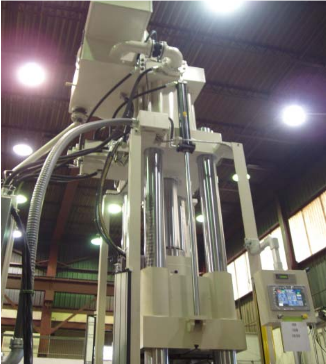
Side view of press showing 10" Allen-Bradley Panel View Plus Touchscreen Control with Keyence Bar Code Scanner attachment.
